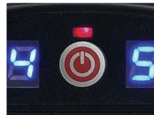
3. The charging LED indicator will illuminate RED when the battery is charging. When the battery is fully charged, the indicator will be BLUE.
